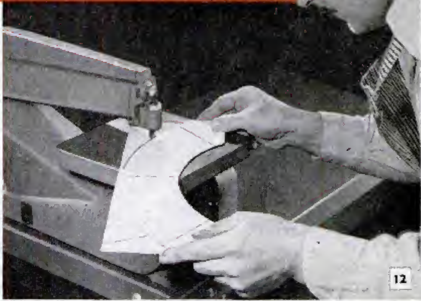
SLITTER AND PORTABLE SHEAR are fast cutters. Both work on the same principle, each having one fixed blade and one moving blade
